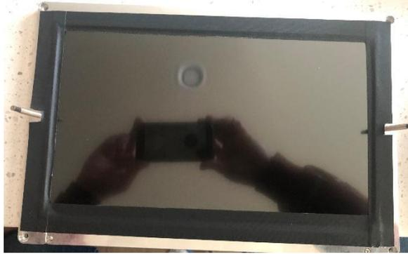
10) Repeat this process for the sides. Using the 2" Tape, cut it to a length longer than the top/bottom of the bezel. Then cut the tape down the center, making two 1" pieces. Be sure to also cut a notch that goes around the VAT mounting screws. Just overlapping the top and bottom glass, secure the tape into place. I have included links to both Bookbinding tape and Electrical Tape, both are good solutions, it is a matter of personal preference.
