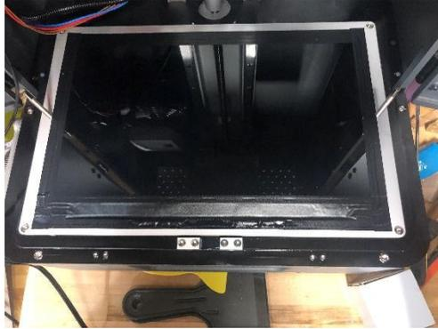
(Note: There was some resin remnants around the original bezel, a plastic putty knife was used as leverage for lifting the bezel gently to remove it)
