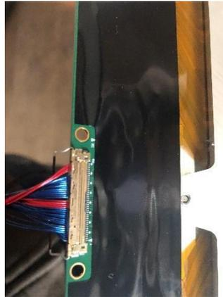
13) Connect the Ribbon Cable to the Driver board. It is very important to note that the cable will fit both ways, but will only correctly display if the correct pins are lined up. Make sure the cable is connected as in the picture below. Black dot side of the cable to the driver board.
